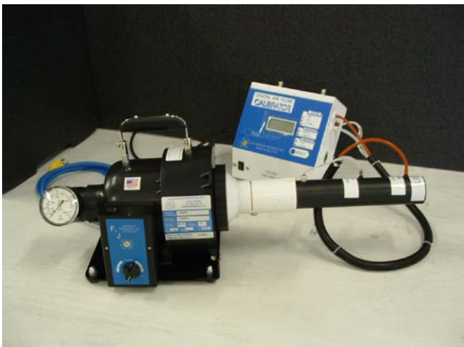
Calibration Setup for Portable High Volume Air Sampler with 4" (102mm) D Filter Holder
